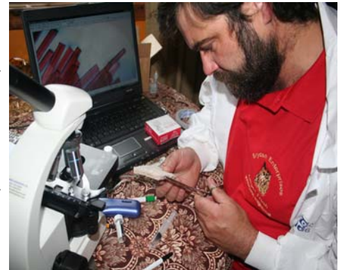
John carrying out fiber analysis during the investigation of a carpet fault
